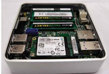
The answer to these problems lies in the Akasa Tesla H case, which is specifically designed for the latest NUC. It's a passively cooled model that adds two 2.5."
